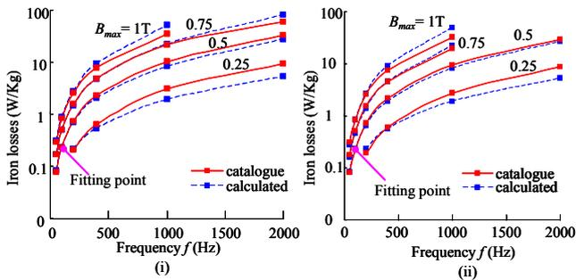
Fig. 4. Comparison of calculated iron losses with catalogue data taking account of skin effect of oriented materials (i) 23P90,  $k_e = 2.92$ , (ii) 23P110,  $k_e = 2.38$ .
