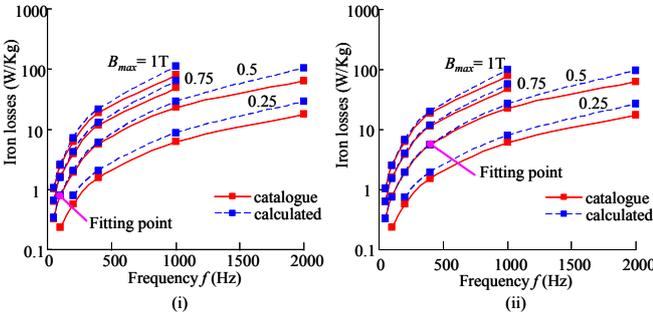
Fig. 3. Comparison of calculated iron losses with catalogue data not taking account of skin effect of non-oriented materials (i) 35A270,  $k_e = 1.94$ , (ii) 35A440,  $k_e = 1.75$ .
