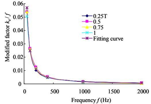
Fig. 6. Variation of modified factor  $k_e$  with maximum average flux density  $B_{max}$  and frequency  $f$ . (oriented material: 23P90).
