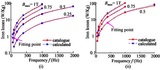
Fig. 2. Comparison of calculated iron losses with catalogue data taking account of skin effect of non-oriented materials (i) 35A270,  $k_e = 1.62$ , (ii) 35A440,  $k_e = 1.45$ .
