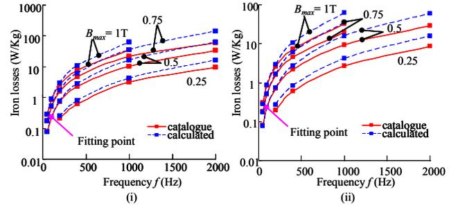
Fig. 5. Comparison of calculated iron losses with catalogue data not taking account of skin effect of oriented materials (i) 23P90,  $k_e = 2.66$ , (ii) 23P110,  $k_e = 2.57$ .
