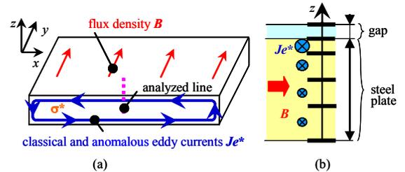
Fig. 1. Modelling method of modifying conductivity taking account of skin effect, (a) modelling, (b) mesh for half region of one steel plate.
